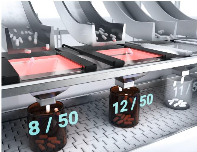
Array fiber optics are used for position-independent detection of irregular objects. Unlike fiber optics with a single, point-shaped light beam, array fiber optics generate a broad, linear light band. Depending on the width of the array fiber optics and the operating principle, the maximum detection
