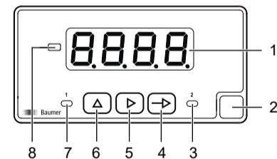
After power on the device is in **RUN** mode. The current value (actual value) is displayed.
