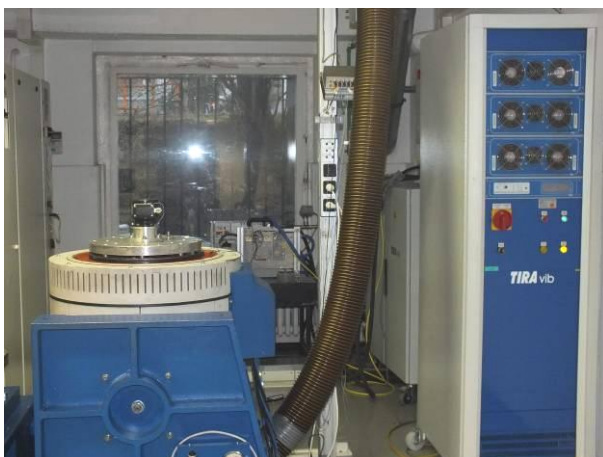
picture 5 Incremental Encoder POG 10 specimen on the vibration test device during vibration test in Z-axis
