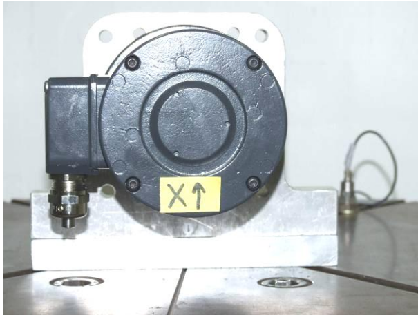
picture 7 Incremental Encoder POG 10 on the shock table with acceleration sensor during shock test in X-axis, positive direction
