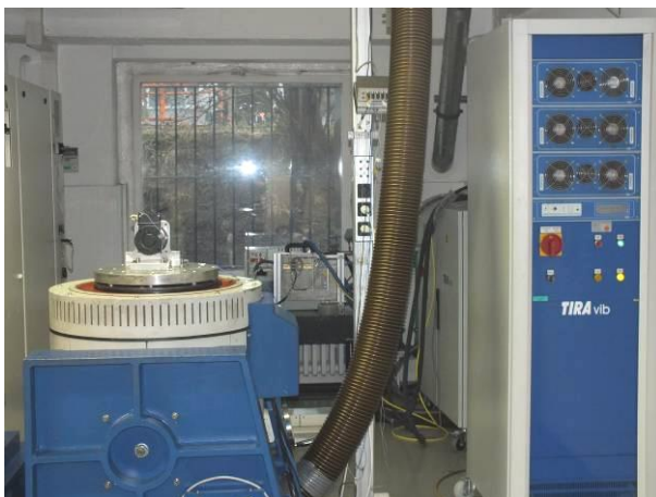
picture 3 Incremental Encoder POG 10 specimens on the vibration test device during vibration test in Y-axis
