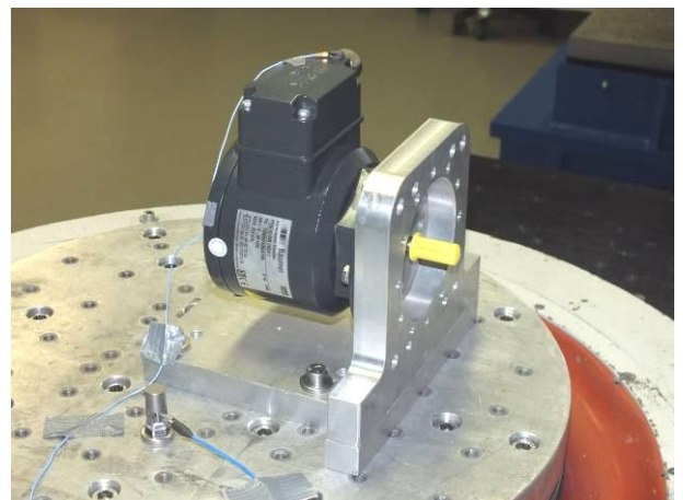
picture 4 Incremental Encoder POG 10 on the vibration table with acceleration sensors during vibration test in Y-axis
