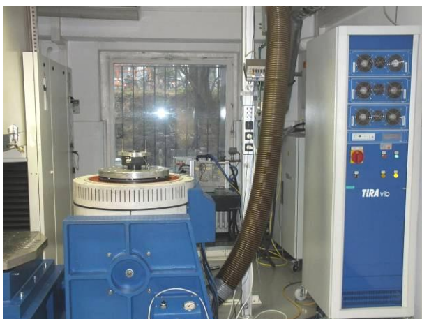
picture 5 Incremental Encoder HOG 16 specimen on the vibration test device during vibration test in Z-axis
