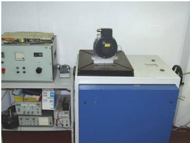
picture 9 Incremental Encoder HOG 16 on the shock table with acceleration sensor during shock test in Y-axis, positive direction
