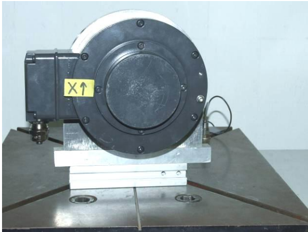
picture 7 Incremental Encoder HOG 16 on the shock table with acceleration sensor during shock test in X-axis, positive direction
