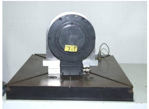
picture 10 Incremental Encoder HOG 16 on the shock table with acceleration sensor during shock test in Y-axis, negative direction
