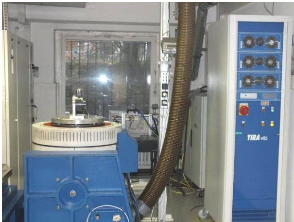
picture 3 Incremental Encoder HOG 16 specimens on the vibration test device during vibration test in Y-axis
