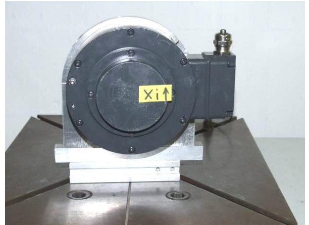
picture 8 Incremental Encoder HOG 16 on the shock table with acceleration sensor during and shock test in X-axis, negative direction
