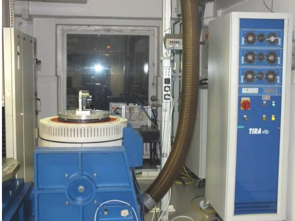
picture 1 Incremental Encoder HOG 16 on the vibration test device during vibration test in X-axis
