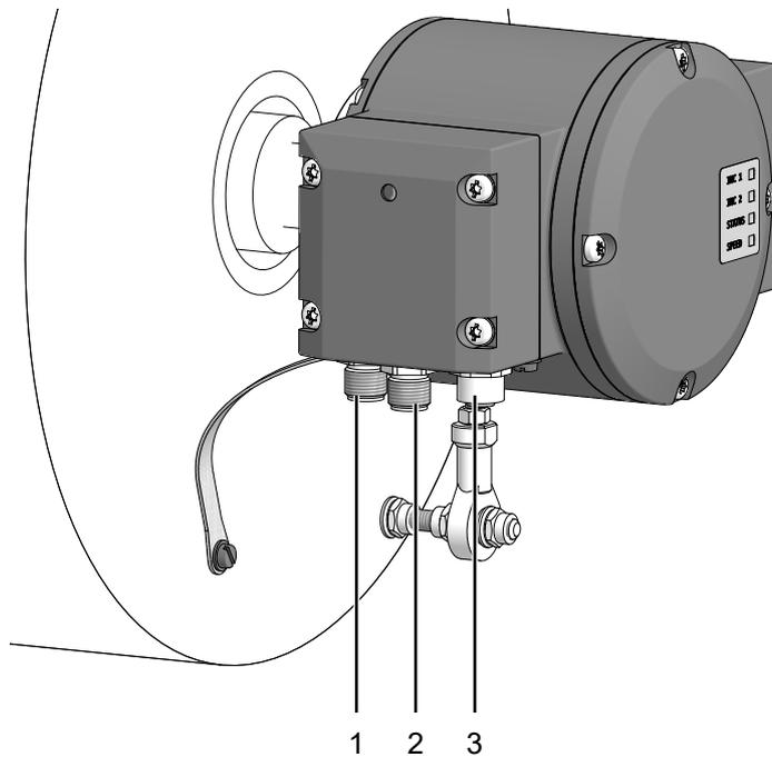
Abb. 5: Anschlüsse HMG10 Profibus DP
