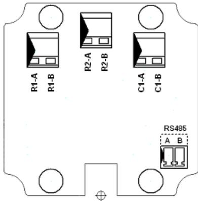
Fig. 18: DSL.E terminal assignments
