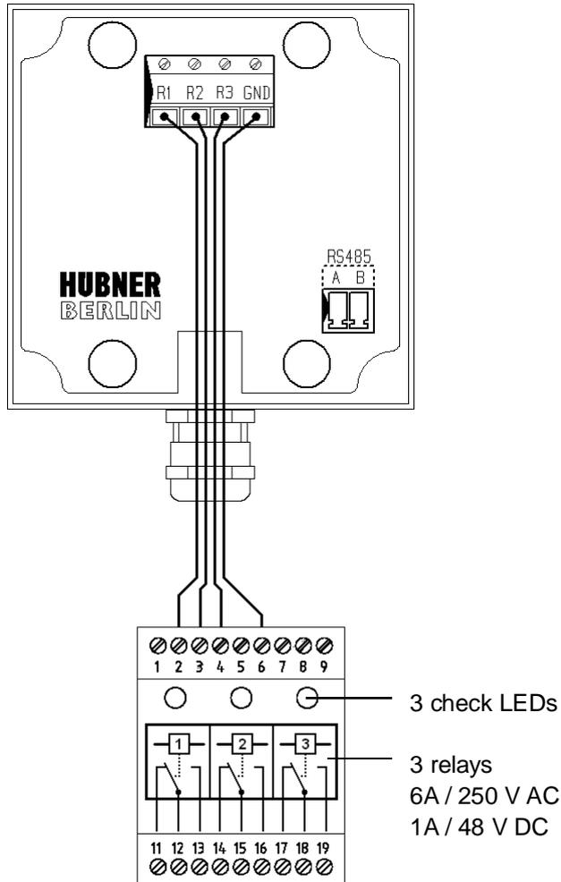
Fig. 20: Connections for DS 93 R
