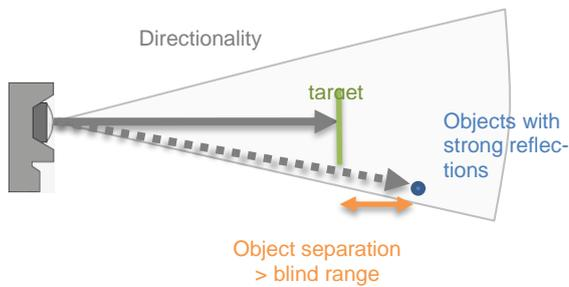
**Fig 8** Separate strongly reflecting objects from target
