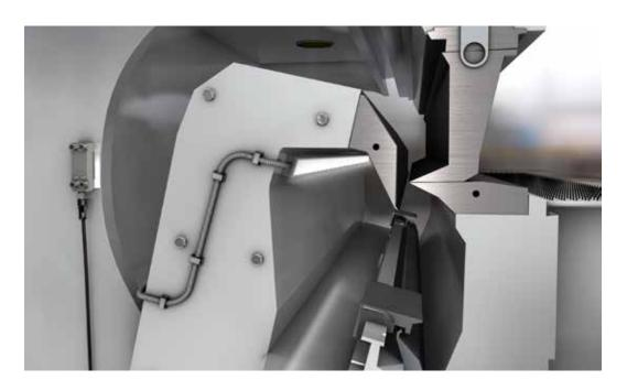
In the bending unit, the DSRT strain sensor monitors the material characteristics of the work pieces throughout the entire process.
