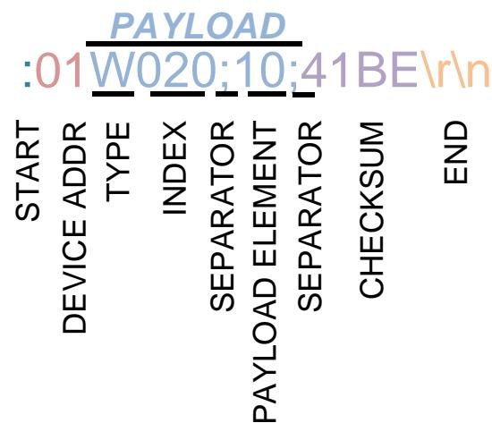
The information to be transmitted is called PAYLOAD and has to be sent in a so-called frame so that the command can be recognized and processed.
