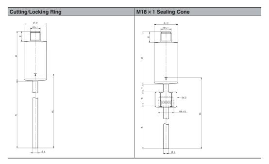
Process connection length PCL in the case of a cutting/locking ring = probe length PL + 9 mm Process connection length PCL in the case of an M18 $\times$ 1 sealing cone = probe length PL + 32 mm
