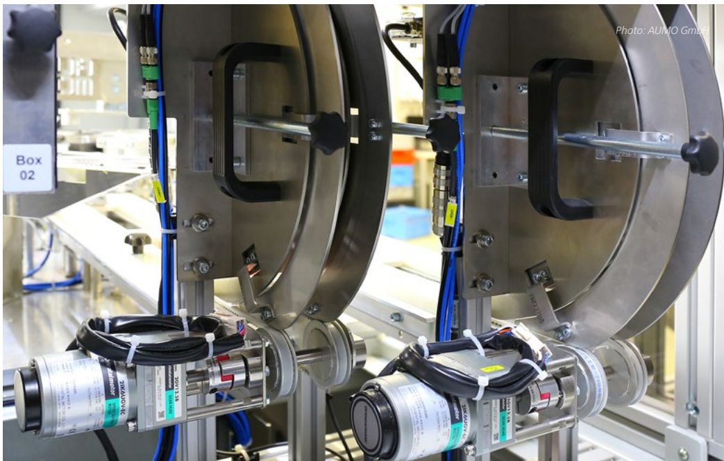
Two rotating units turn the socket plates for back side inspection.
