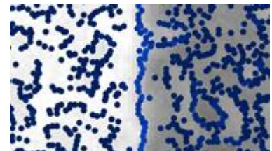
Too many contours (contour recognition sensitivity must be increased)
