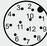
Power Supply / Digital-IOs (on camera side) (SACC-CI-M12MS-12CON-L180) wire colors of the connecting cable (ordered separately)
