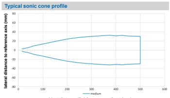
$\begin{tabular}{ll} \textbf{object distance (So) from sensor front (mm)} \\ \textbf{standard target with } 30 \times 30 \ \text{mm, directed rectangular to sensor's reference axis} \\ \end{tabular}$
