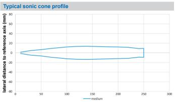
object distance (So) from sensor front (mm) standard target with 15 x 15 mm, directed rectangular to sensor's reference axis
