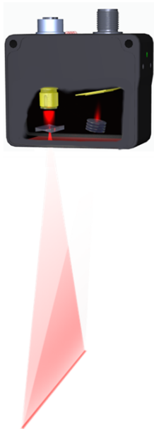
III. 3: Triangulation principle
