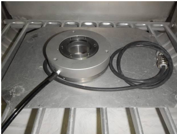
Picture 3 Incremental encoder HOGS151 DN 5000 in the dust chamber SK 160 with overpressure hose before the dust test IP6X
