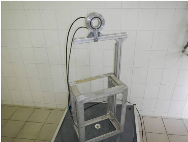
Picture 7 Incremental encoder HOGS151 DN 5000 mounted on the turn table before the protection against splash water test IPX4
