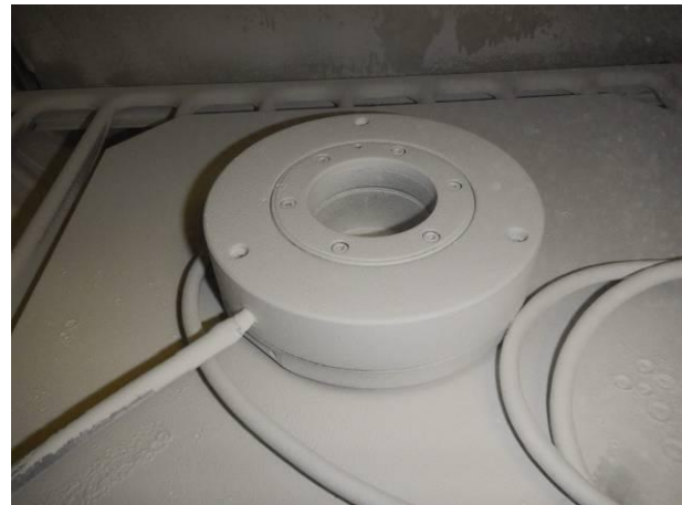
Picture 4 Incremental encoder HOGS151 DN 5000 in the in the dust chamber SK 160 with overpressure hose after the dust test IP6X
