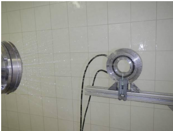
Picture 9 Incremental encoder HOGS151 DN 5000 with standardized splash water during the protection against splash water test IPX4
