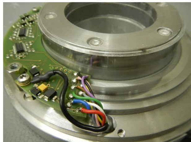
Picture 6 Incremental encoder HOGS151 DN 5000 without visible traces of dust inside after the dust test IP6X
