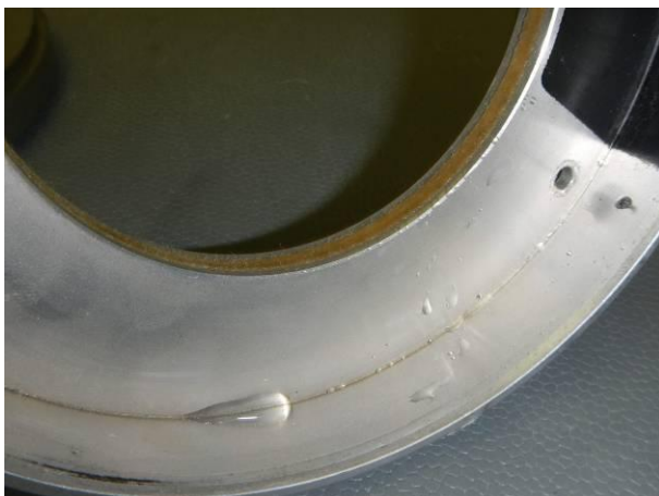
Picture 11 Incremental encoder HOGS151 DN 5000 with visible traces of water inside the housing after the protection against splash water test IPX4
