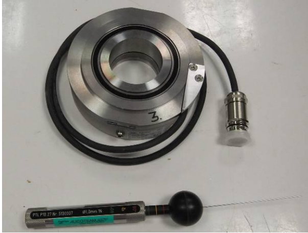
Picture 1 Incremental encoder HOGS151 DN 5000 with standardized test wire (Ø 1 mm, 1 N) before the access to hazardous parts test IP6X
