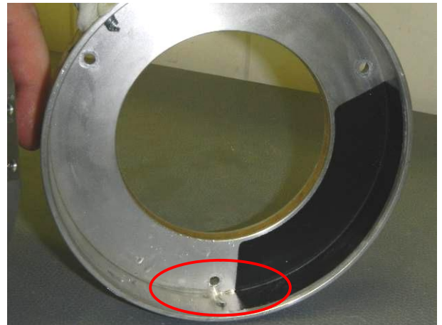
Picture 10 Incremental encoder HOGS151 DN 5000 with visible traces of water inside the housing after the protection against splash water test IPX4
