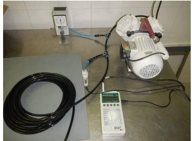
Picture 8 Incremental encoder HOGS151 DN 5000 with equipment for overpressure regulation before the protection against splash water test IPX4
