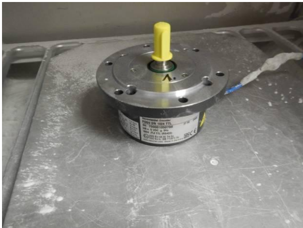
Picture 3 Incremental encoder FOG9 DN 1024 TTL in the dust chamber SK 160 before the dust test IP6X
