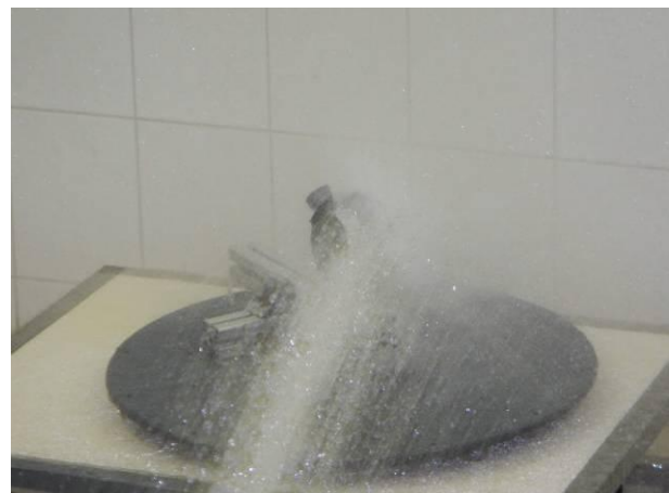
Picture 6 Incremental encoder FOG9 DN 1024 TTL on the turn table with standardized water jet during the protection against water jets test IPX6
