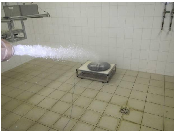
Picture 5 Incremental encoder FOG9 DN 1024 TTL on the turn table with standardized water jet during the protection against water jets test IPX6
