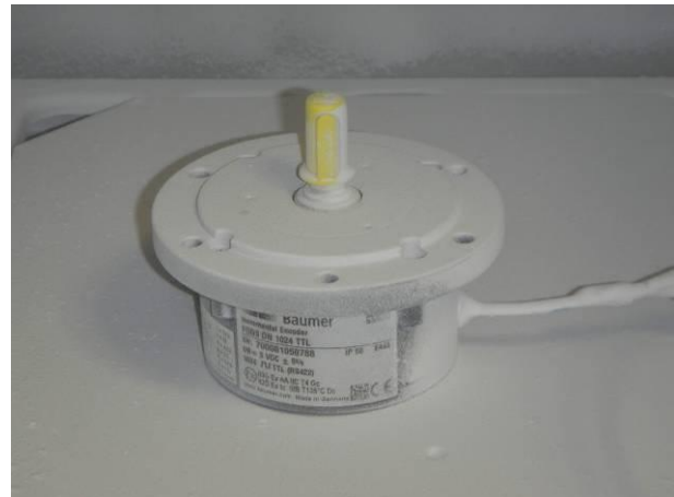
Picture 4 Incremental encoder FOG9 DN 1024 TTL in the dust chamber SK 160 after the dust test IP6X
