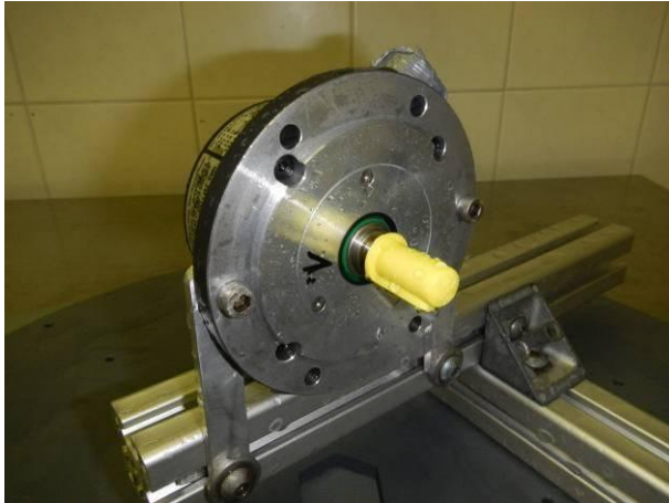
Picture 7 Incremental encoder FOG9 DN 1024 TTL without any alterations after the protection against water jets test IPX6
