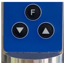
Figure 6: Examples of robust control elements without housing openings
