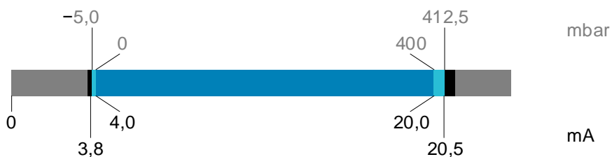
Figure 3: Current signaling range by example of a 400 mbar pressure sensor
